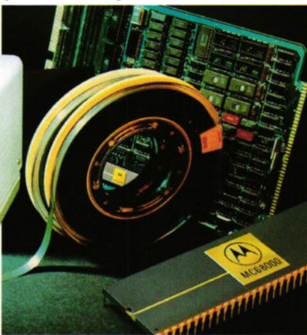
MC68000, Motorola's most powerful microprocessor, with its design module in the background.
